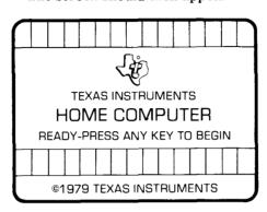
If the computer is ON, hold down the **SHIFT** key and press **Q** to make the master title screen appear. Then slide the module into the slot on the console.
