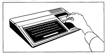
1. *If the computer is OFF,* slide the module into the slot on the console, and turn the computer on. The master title screen should then appear.
