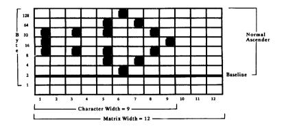
The character is 9 dots wide and is flush to the left. We'll print it in 10 cpi Utility. Just like 8-pin graphics, each byte specifies a dot column, and the value of each byte is determined by adding up the values of its bits.
