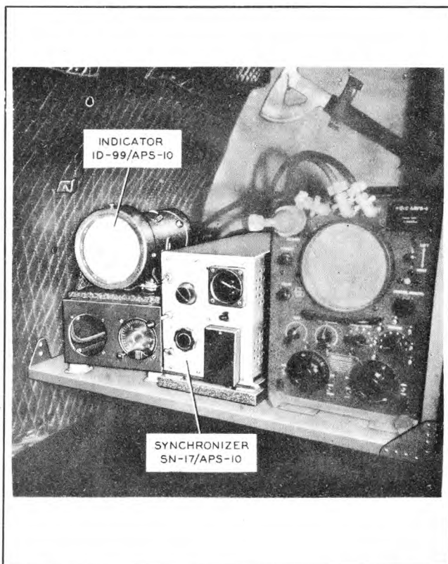
Figure 2-7. Radio Set AN/APS-10—Installation (C-47) Navigator's Compartment, Shelf
