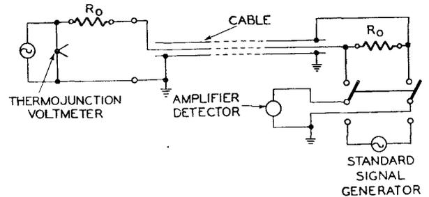
FIG 4 — ARRANGEMENT OF APPARATUS FOR INSERTION LOSS MEASUREMENTS
