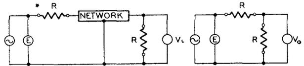
FIG 3 — PRINCIPLE OF INSERTION LOSS MEASUREMENTS
