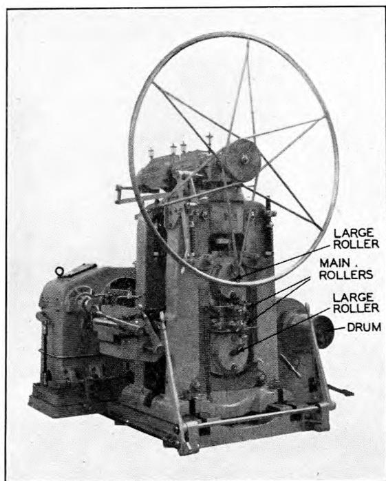
FIG. 3.—"FOUR-HIGH" MILL.
