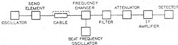
FIG. 6.—DIAGRAMMATIC ARRANGEMENT OF APPARATUS IN FREQUENCY CHANGE METHOD OF INSERTION LOSS MEASUREMENT
