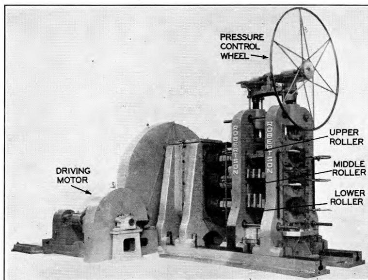
FIG. 2.—"THREE-HIGH" MILL.
