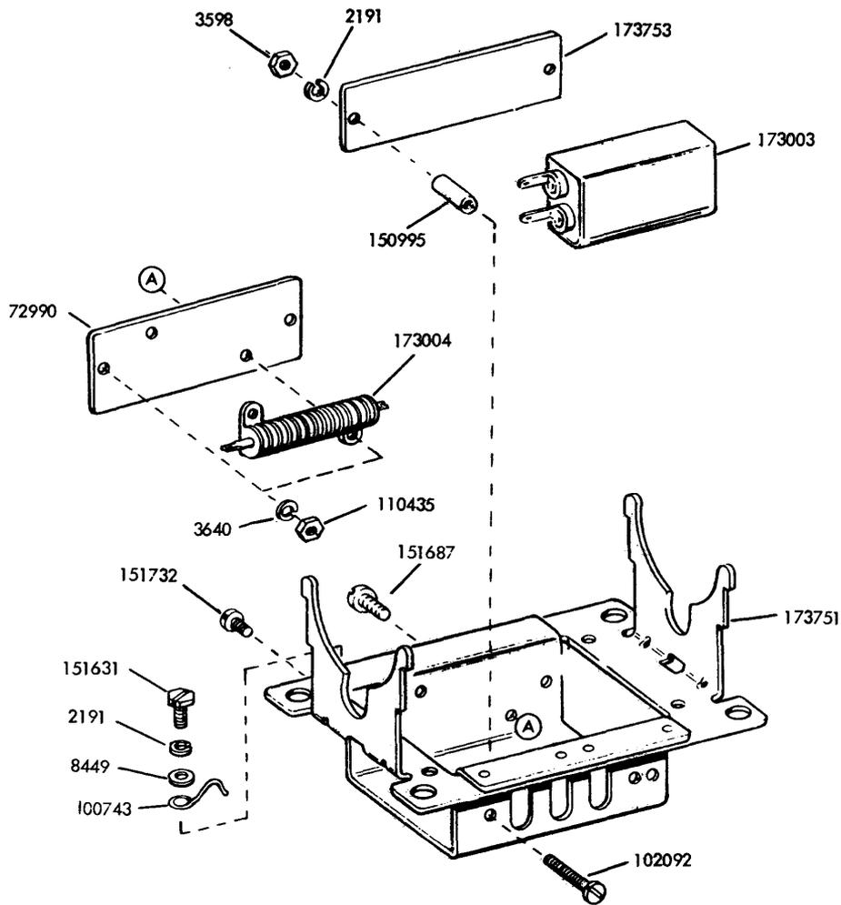
FIGURE 22. SERIES MOTOR MOUNTING PARTS
