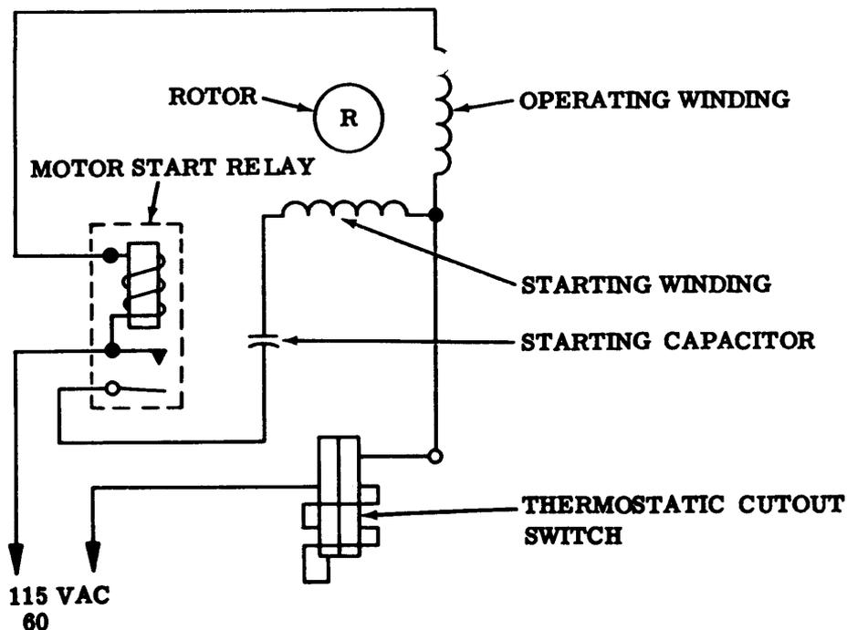
Figure 4 - Typical Synchronous Motor Unit Schematic Diagram
