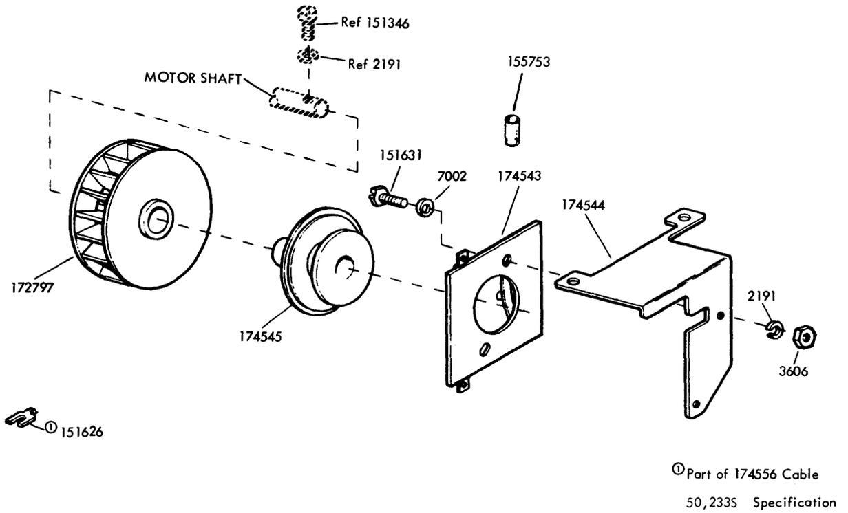
FIGURE 25. 174546 MODIFICATION KIT TO PROVIDE MOTOR RUNNING CONTACTS
