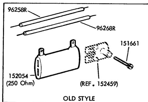
FIGURE 19. SERIES MOTOR MOUNTING PARTS
