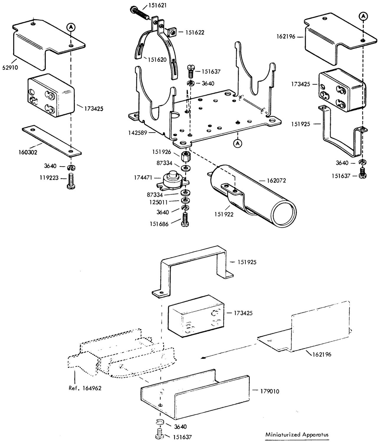
FIGURE 10. RELAY AND CAPACITOR MOUNTING (SYNCHRONOUS)
