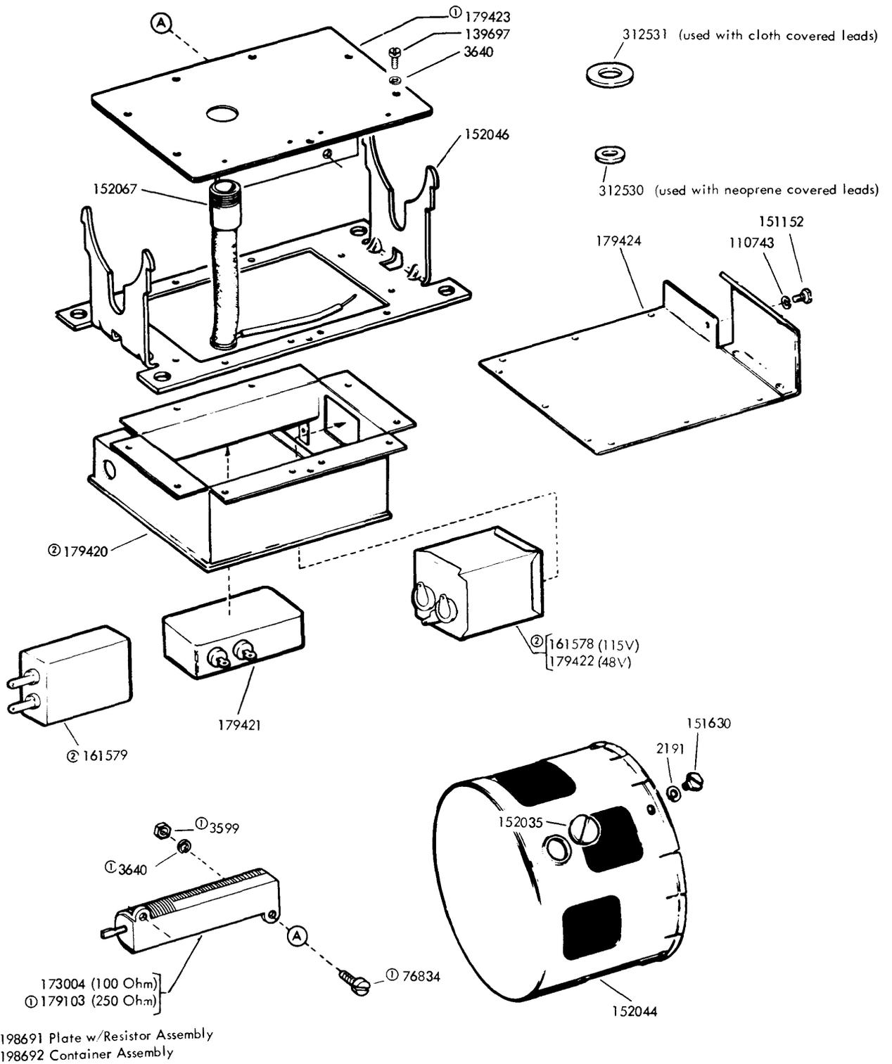
FIGURE 21. SERIES MOTOR MOUNTING PARTS WITH RF SUPPRESSION
