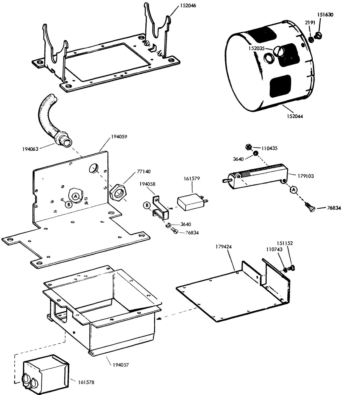
FIGURE 24. SERIES MOTOR MOUNTING PARTS WITH RF SUPPRESSION
