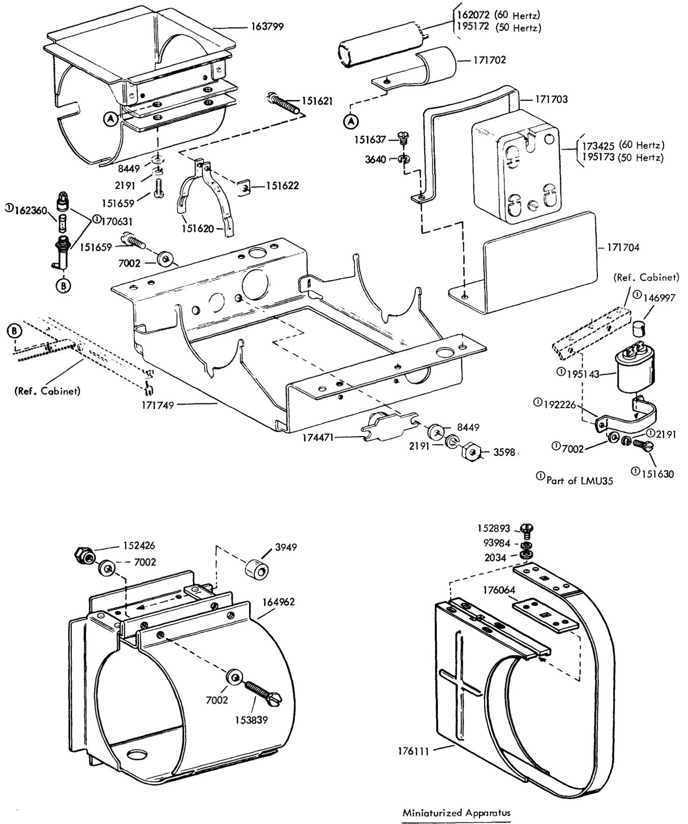
FIGURE 11. RELAY, CAPACITOR MOUNTING AND BRACKET (SYNCHRONOUS)
