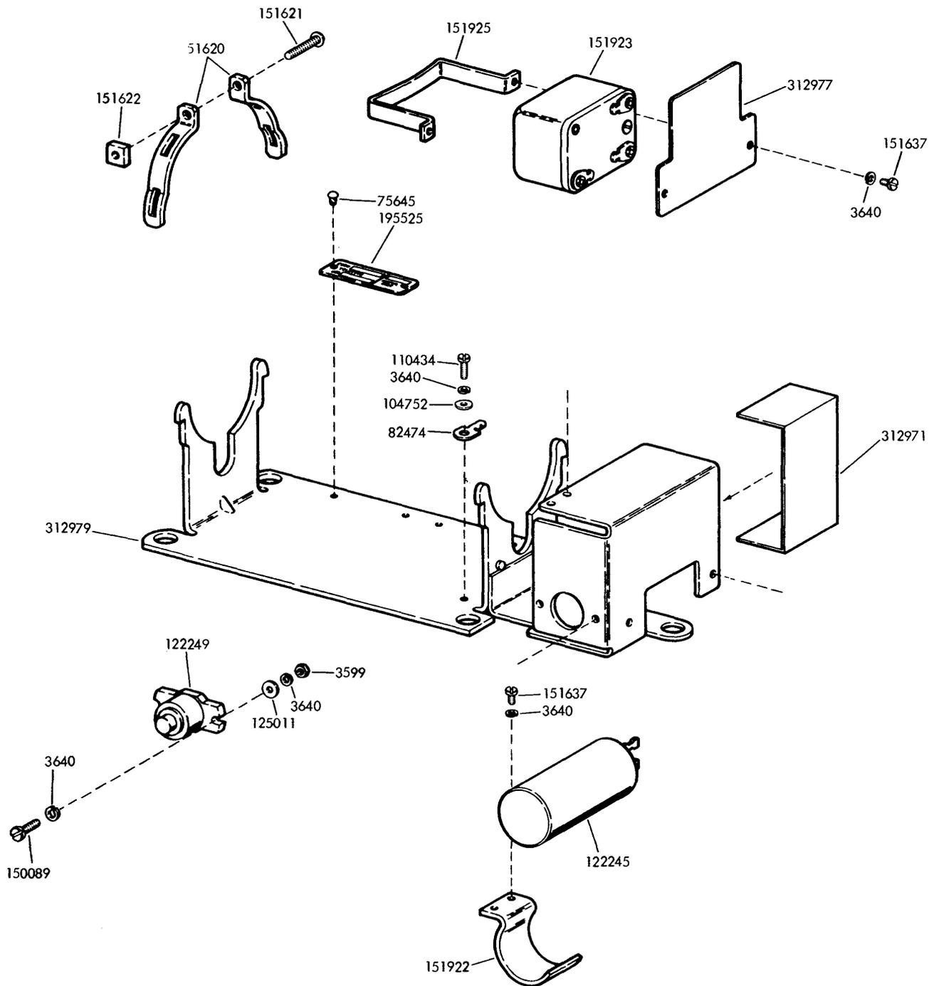
FIGURE 13. RELAY AND CAPACITOR MOUNTING (SYNCHRONOUS)
