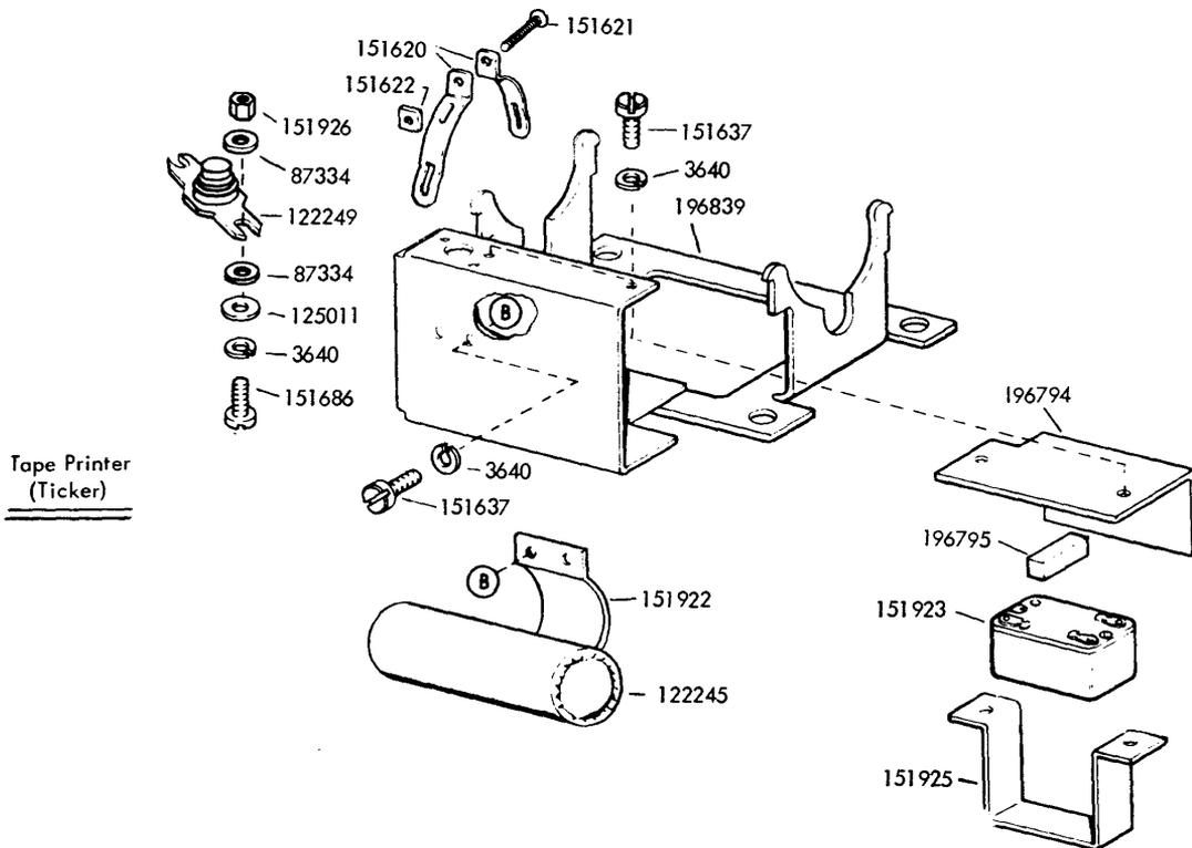
FIGURE 7. RELAY AND CAPACITOR MOUNTING (SYNCHRONOUS)
