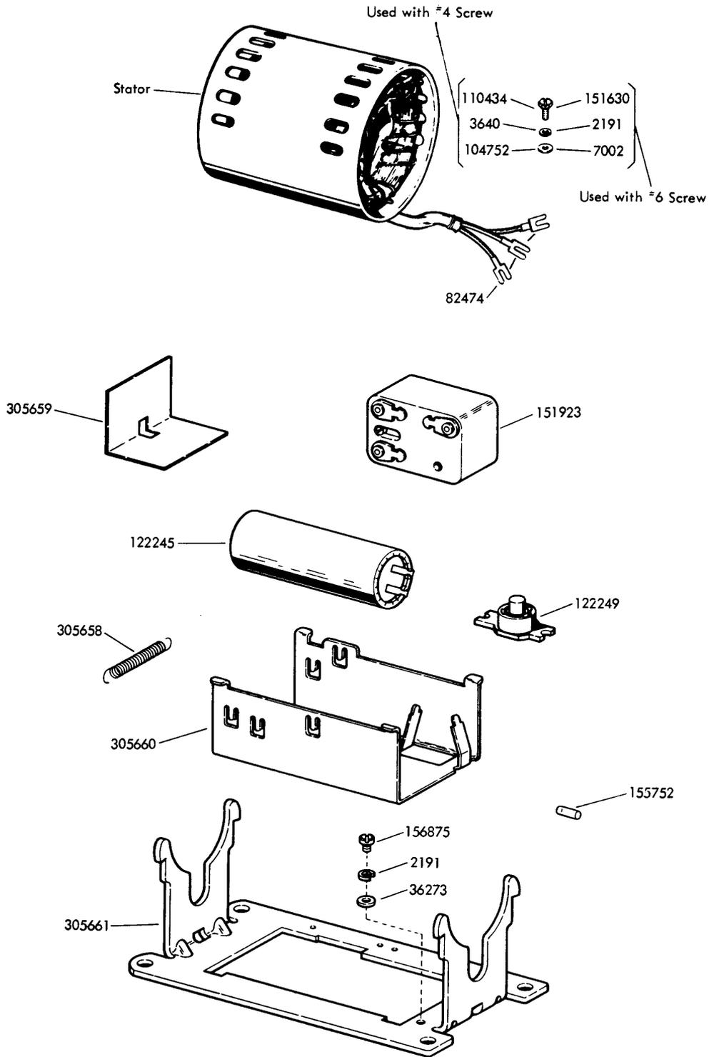
FIGURE 6. RELAY AND CAPACITOR MOUNTING
