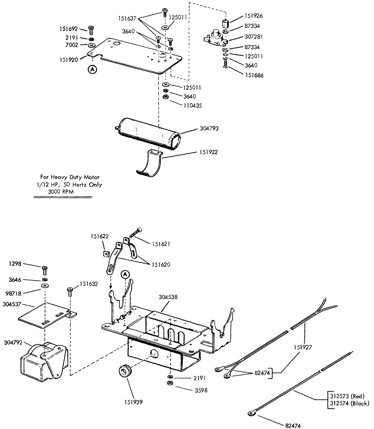
FIGURE 5. RELAY AND CAPACITOR MOUNTING (SYNCHRONOUS)
