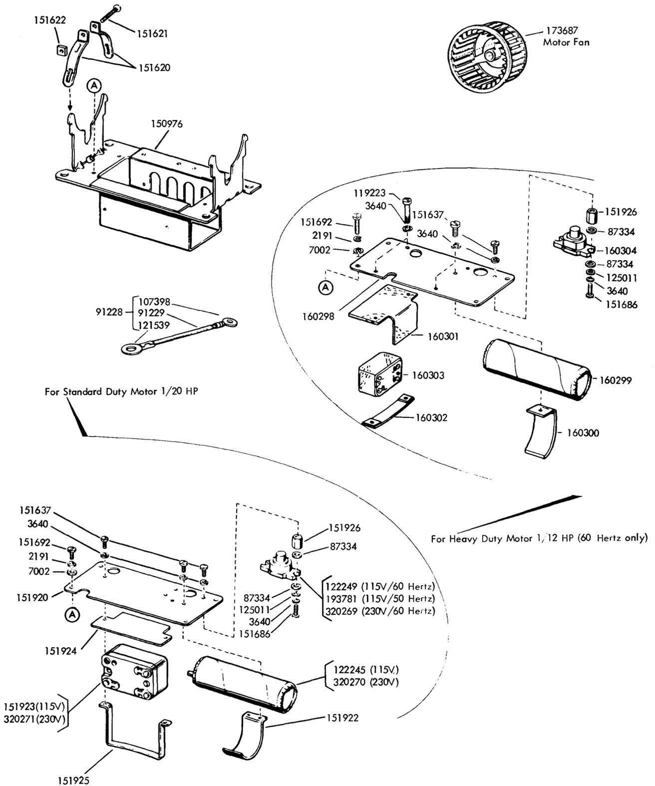
FIGURE 4. RELAY AND CAPACITOR MOUNTING (SYNCHRONOUS)
