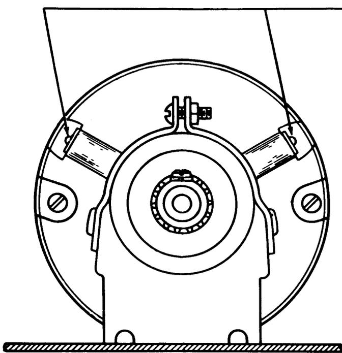
O6 Two Oilers at Each End (Depress Oiler With Metal Object)
