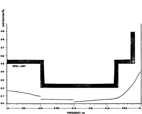
Typical harmonic distortion of LF1, LFP1 and LFM4 when delivering 12V pk-pk into  $600\Omega$  over range 10Hz to 100kHz
