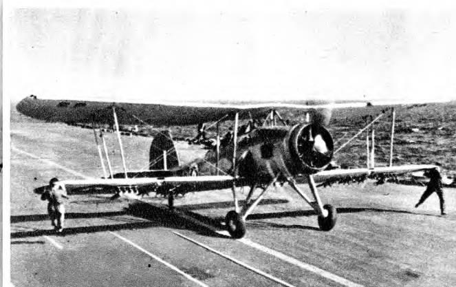
7 The pilot taxis forward, and the wings are folded back by the "pin party," so that the aircraft can descend in the lift shaft.
