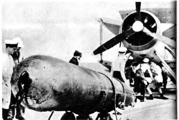
SWORD OF THE SWORDFISH. One of the Ark's torpedoes is wheeled under the Swordfish's fuselage, where it is jacked into the dropping position.
