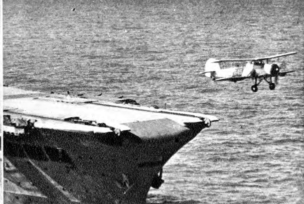
2 With the carrier dead into wind, as the steam jet set for'ard in the deck shows, a Swordfish flies off.
