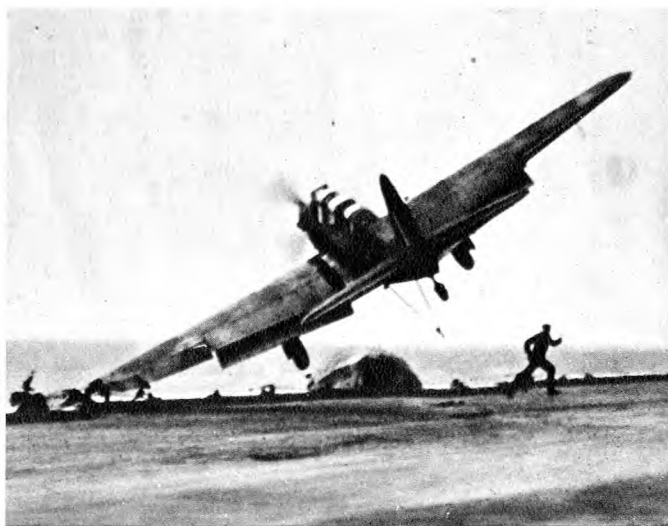
FULMAR IN TROUBLE. Flying from carriers is not easy, and risks have to be run. This Fulmar missed the landing wires, began to take off again, banked too steeply, and caught its wing tip. The crew of two were both flung clear and rescued unhurt from the water.
