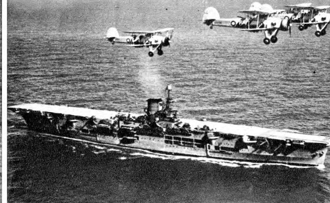
3 All now in the air and in formation, the aircraft circle round the carrier. They must land on from astern and into wind.
