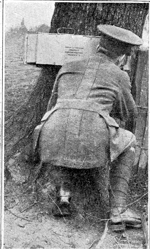
The periscope can be used horizontally. How an enemy is observed by an operator in hiding behind a tree.
