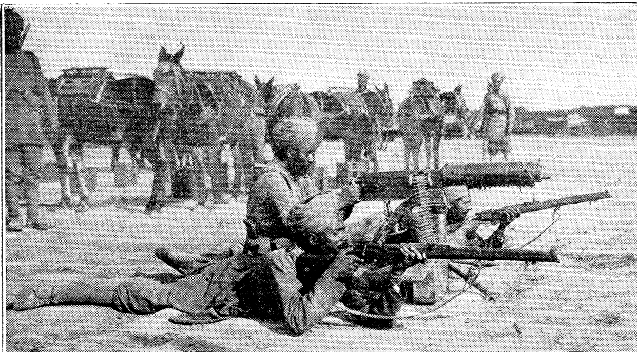
Sikhs working a Maxim gun. This is one of the most generally used guns, and capable of firing about 450 rounds a minute. The belt of cartridges is seen passing through the feed-block while the gunner directs the fire by means of two handles at the rear.
