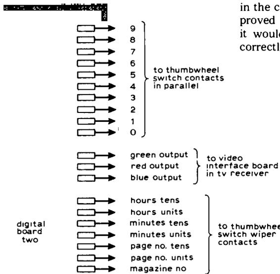
Fig. 5. Function switching. The "CLEAR" switch is a push, non-locking type, the "TIME" button is a push-push, locking switch and the rest are interlocking. Further constructional information appears in the next article.
