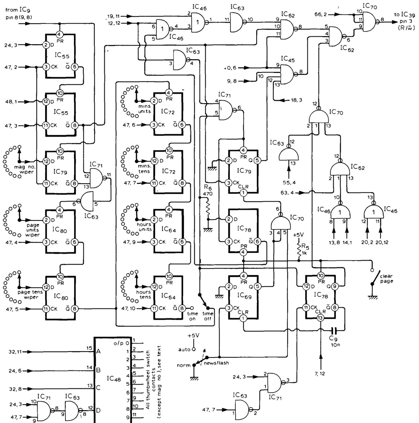
It will be noticed from the circuit diagram that the clear input of IC<sub>79</sub> is fed from the output of (70, 6). However, this only has any effect in the auto-newsflash mode of operation which will be dealt with later. During normal operation the clear input is held at 1 because one input of (70, 6) is held at 0 by the auto/normal switch.
