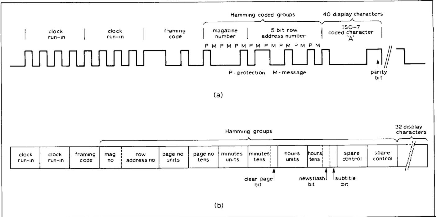
Fig. 4. Layouts of typical rows of data bits. A display row (row 5 of magazine 1) is shown at (a) and at (b) is a page-header row.
