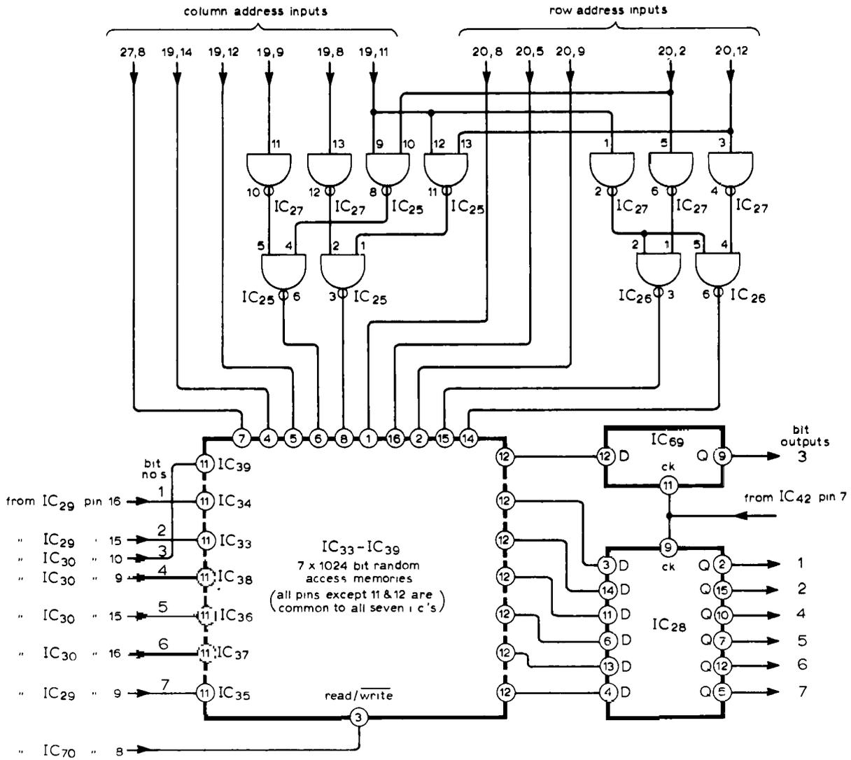
Fig. 4. Circuit diagram of the code converter and data store. IC<sub>25,26</sub> are 7400, IC<sub>27</sub> is 7404, IC<sub>28</sub> is a 74174, IC<sub>69</sub> is a 7474 and the r.a.m.s are 2602B or 2102B.
