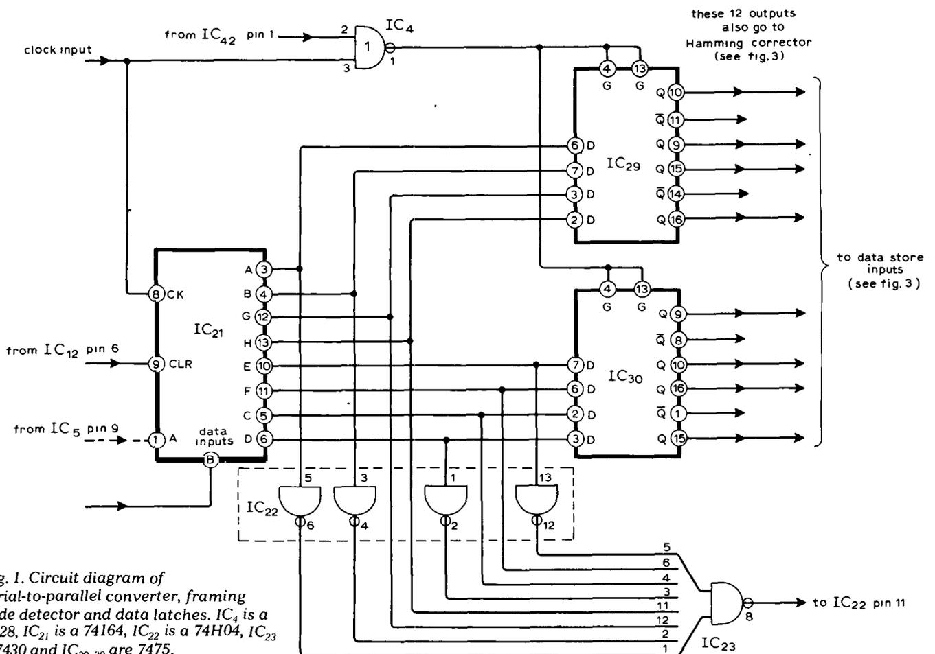
Fig. 1. Circuit diagram of serial-to-parallel converter, framing code detector and data latches. IC<sub>4</sub> is a 7428, IC<sub>21</sub> is a 74164, IC<sub>22</sub> is a 74H04, IC<sub>23</sub> a 7430 and IC<sub>29,30</sub> are 7475.
