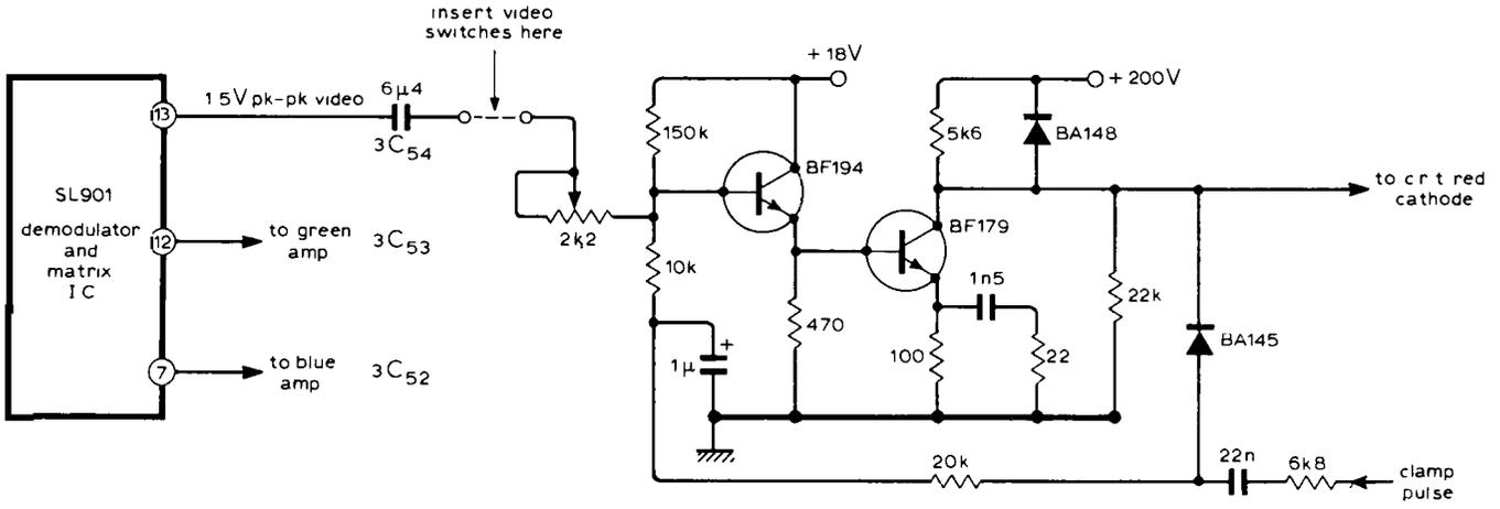
Fig. 2 Video output circuitry of the Bush CTV182S, CTV184S and CTV187CS
