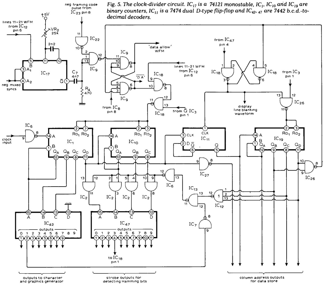
Fig. 5. The clock-divider circuit. IC<sub>17</sub> is a 74121 monostable, IC<sub>1</sub>, IC<sub>10</sub> and IC<sub>19</sub> are binary counters, IC<sub>11</sub> is a 7474 dual D-type flip-flop and IC<sub>42</sub>, 47 are 7442 b.c.d.-to-decimal decoders.
