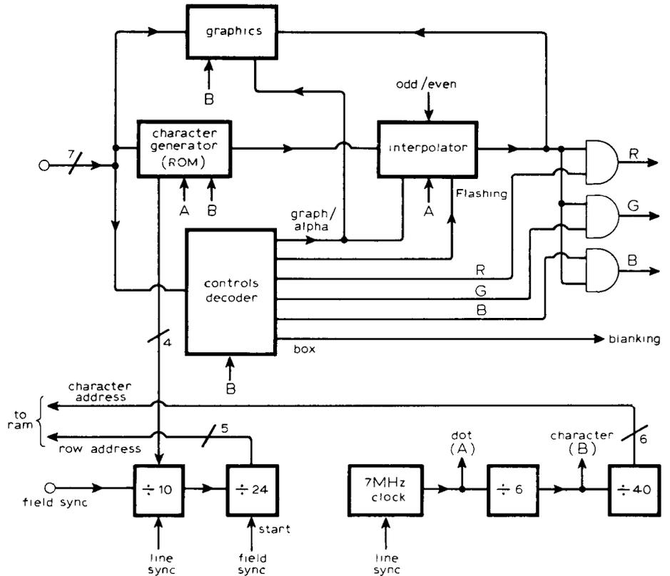
Fig. 8. A typical output processor.
