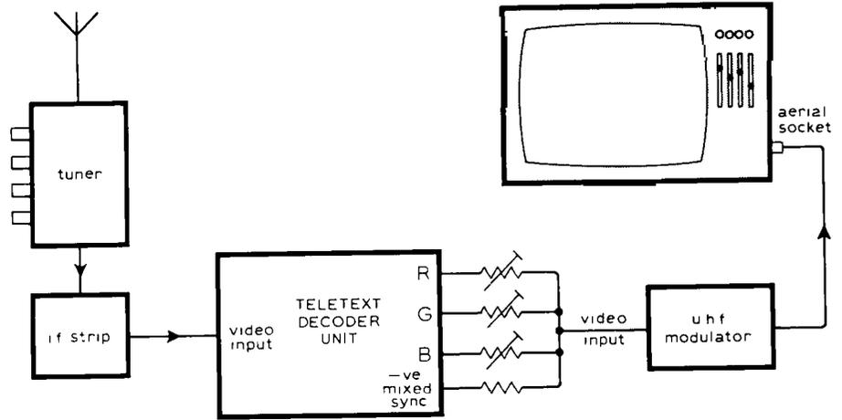
Fig. 3. Alternative arrangements for rented television sets. This has the disadvantage that only a black and white display will be obtained.
