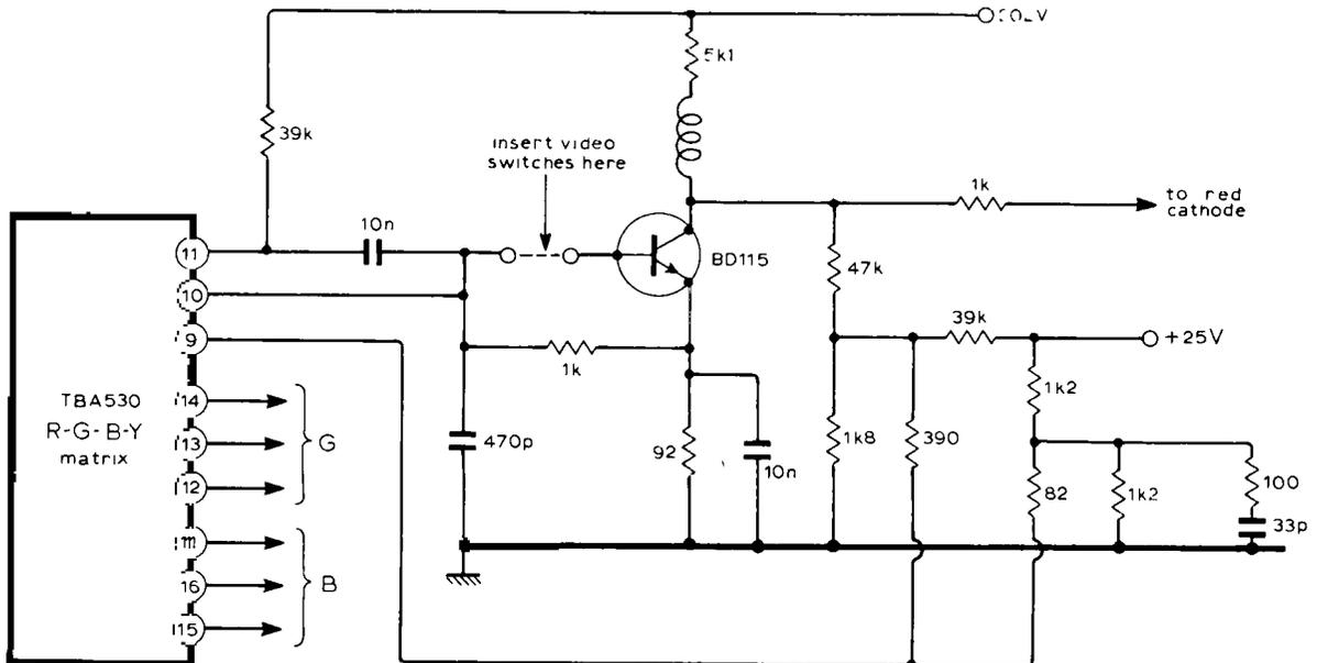
should be noted that the polarity of these and the input electrolytics will depend on the individual receiver design and may, not be as shown.) Figure 1 shows a fourth pair of switches which are not required when modifying a receiver of the type described. They are useful, however, when modifying a set which has colour-difference amplifiers (R-Y, G-Y and B-Y), as they can be used to switch off the luminance signal, which would otherwise be present while watching the Teletext display.
